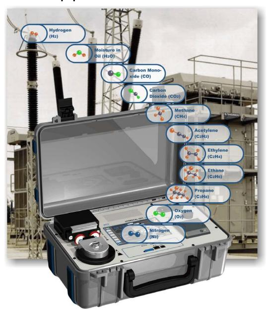
The HYDROCAL 1011 genX P is a portable device for the analysis of dissolved and free gases from the isolation fluid of oil-filled power transformers and other electrical equipment. It individually measures moisture in oil ( $H_2O$ ) and the key gases hydrogen ( $H_2$ ), carbon monoxide (CO), carbon dioxide ( $CO_2$ ), methane ( $CH_4$ ), acetylene ( $C_2H_2$ ), ethylene ( $C_2H_4$ ), ethane ( $C_2H_6$ ), oxygen ( $O_2$ ), nitrogen ( $O_2$ ) and propane ( $O_3$ ) dissolved in transformer oil.
